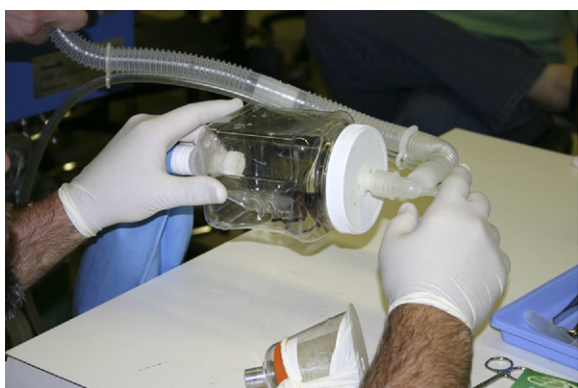
FIGURE 2. An anesthetic induction chamber constructed from a plastic container attached to inflow and outflow hoses. The animal (a tarantula in this image) is placed within the chamber and anesthetic gas is applied accordingly. Photograph courtesy of Michele Mehalick.
